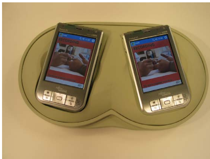
Figure 16: Placed in the docking station the display turns into a two state interface allowing just for pause/record of recording process
