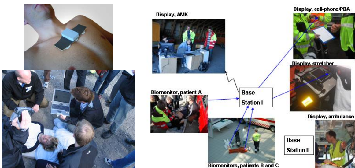
Figure 2 A wireless biomonitor prototype, its data inspected on a ‘wearable’ display.
